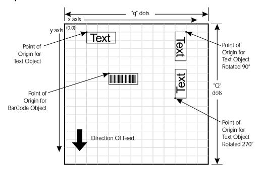
The minimum non printing margin on all edges of the label is 1mm. Printing closer than 1mm to the top or bottom edge of the label may cause the printer to advance unwanted labels or cause the printer to go into error condition.
