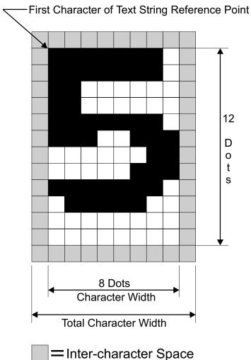
Control text height (in horizontal dots) and width (in vertical dots) with the horizontal and vertical multipliers. The text is oriented first and then the A command's font multipliers are applied.
