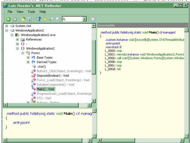
What you see here is reflector and on the right the disassembly of some procedure called Main(): Void, You can see the IL instructions in the disassembly here:
