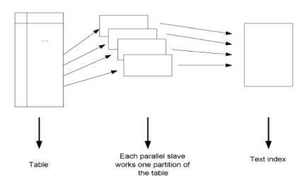
Figure 2: Creating a text index in parallel
