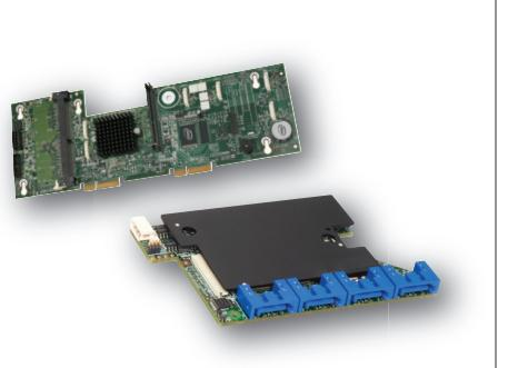
A photograph of two Intel Integrated Server RAID system boards. One is a green board with a large heat sink, and the other is a smaller black board with blue SAS/SATA connectors.
