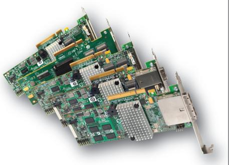
A photograph of two Intel RAID Controllers adapter cards. They are green printed circuit boards with multiple gold-plated edge connectors for installation into server expansion slots.
