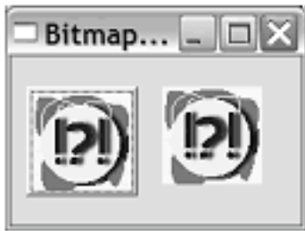
Figure 7.5 A demonstration of a basic bitmap button. The left button is drawn with a 3D effect.
