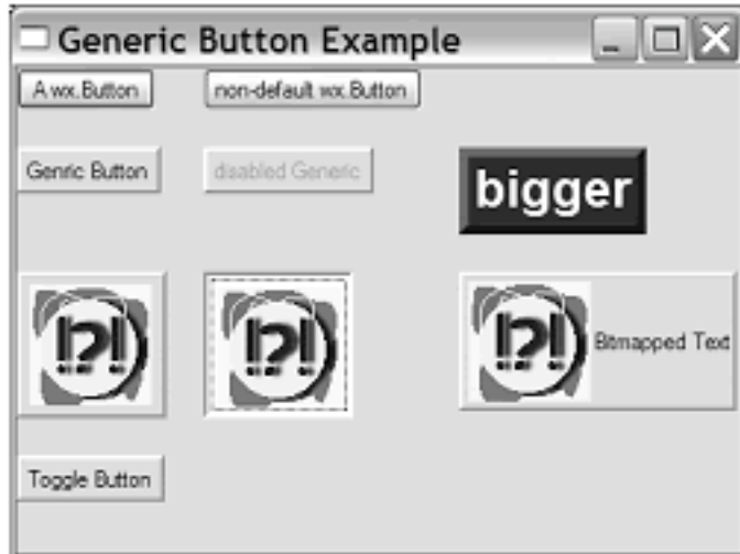
Figure 7.6 Generic buttons. The top row has regular buttons for contrast. This shows different color combination, bitmap, bitmap toggle, and bitmap text buttons.
