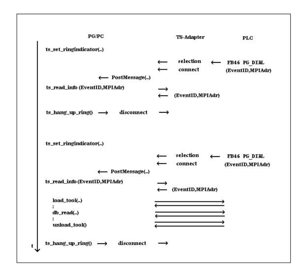
After the TeleService connection has been established successfully, the user can establish a connection to the PLC connected to the TS adaptor using the **load\_tool** function. It is possible to use any amount of PRODAVE functions. This is followed by closing the connection to the PLC using the **unload\_tool** function and closing the TeleService connection by means of **ts\_hang\_up\_dial** or **ts\_hang\_up\_ring**.
