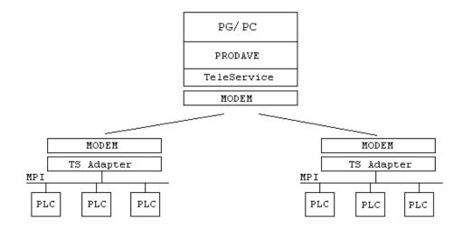
When the TeleService functions are in use it is important to note that the PG/PC interface in system control the module parameter assignment is set to TS-Adaptor
