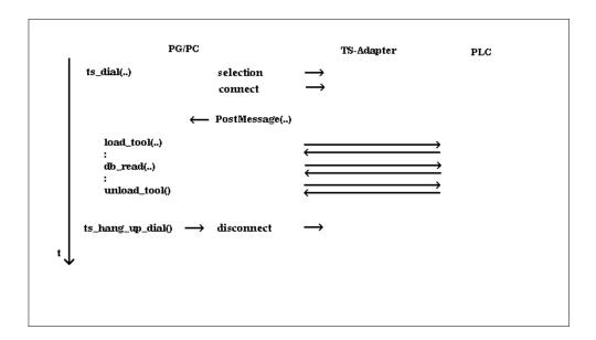
When access protection is activated the TS-Adapter checks the specified password. Providing the password is correct, the connection is established either immediately or after re-dialling from the TeleService Adapter (depending on TeleService parameterisation).
