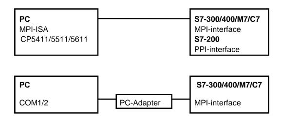
Installation and set-up of the required hardware is carried out via the STEP7-Tool **PG/PC interface parameterisation**, which is available in the system after successful installation.
