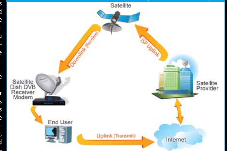
Exhibit 1. Unidirectional Access with Terrestrial Return (also known as Satmodem) 8
