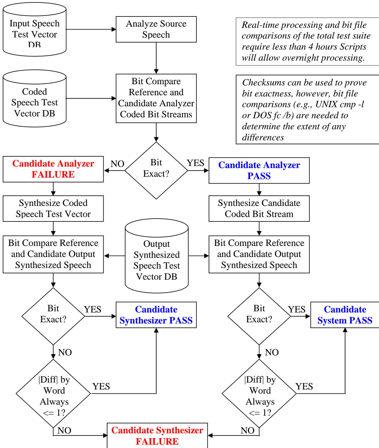
Figure B-1. Test Process Flow for STANAG 4591 Voice Coders
