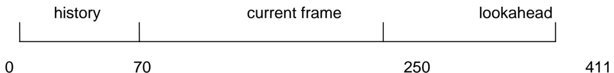
**Figure D-1. The buffer structure of standard 2400 bit/s MELPe coder**
