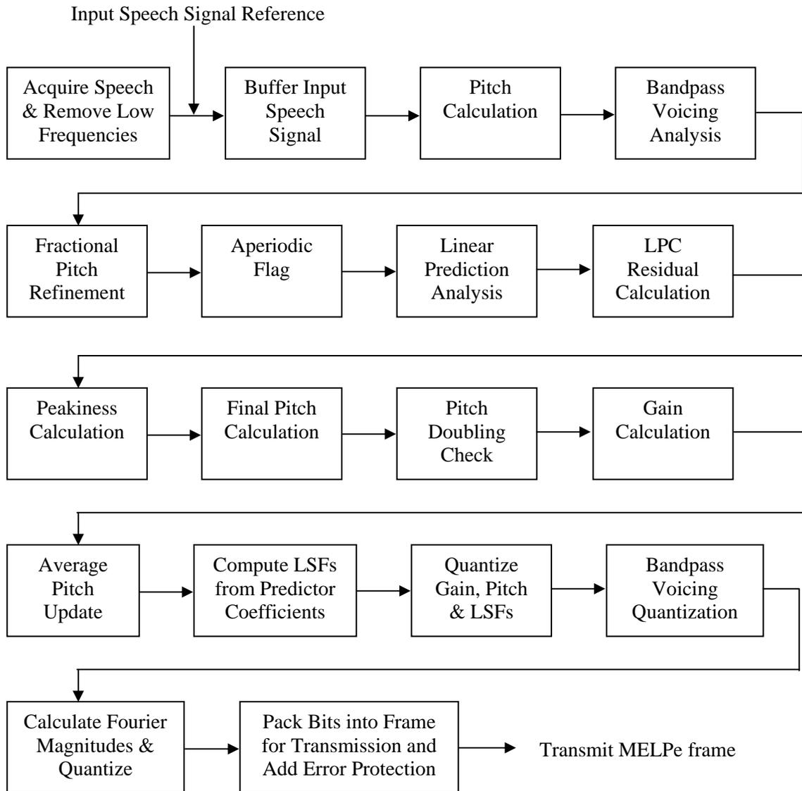
Figure A-1a. MELPe Coder Block Diagram
