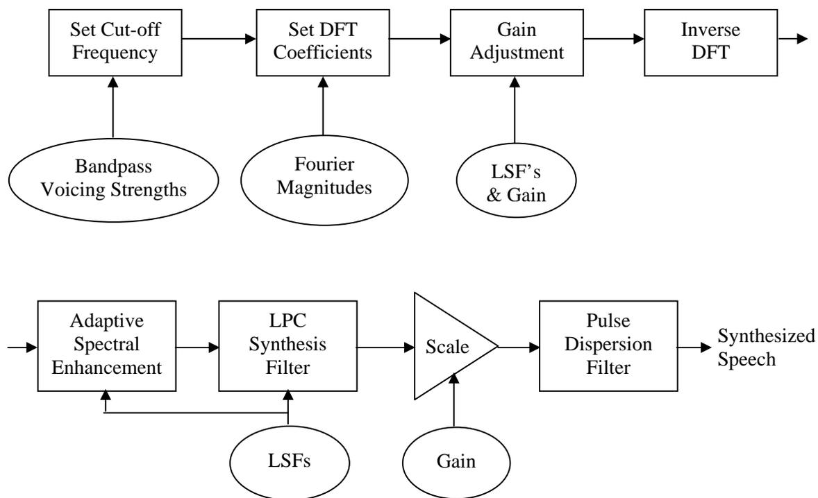
**Figure A-1b. MELPe Decoder Block Diagram**
