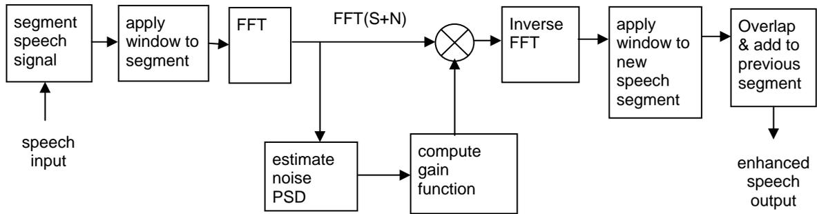
**Figure E-1. Top Level View of Noise Preprocessor**
