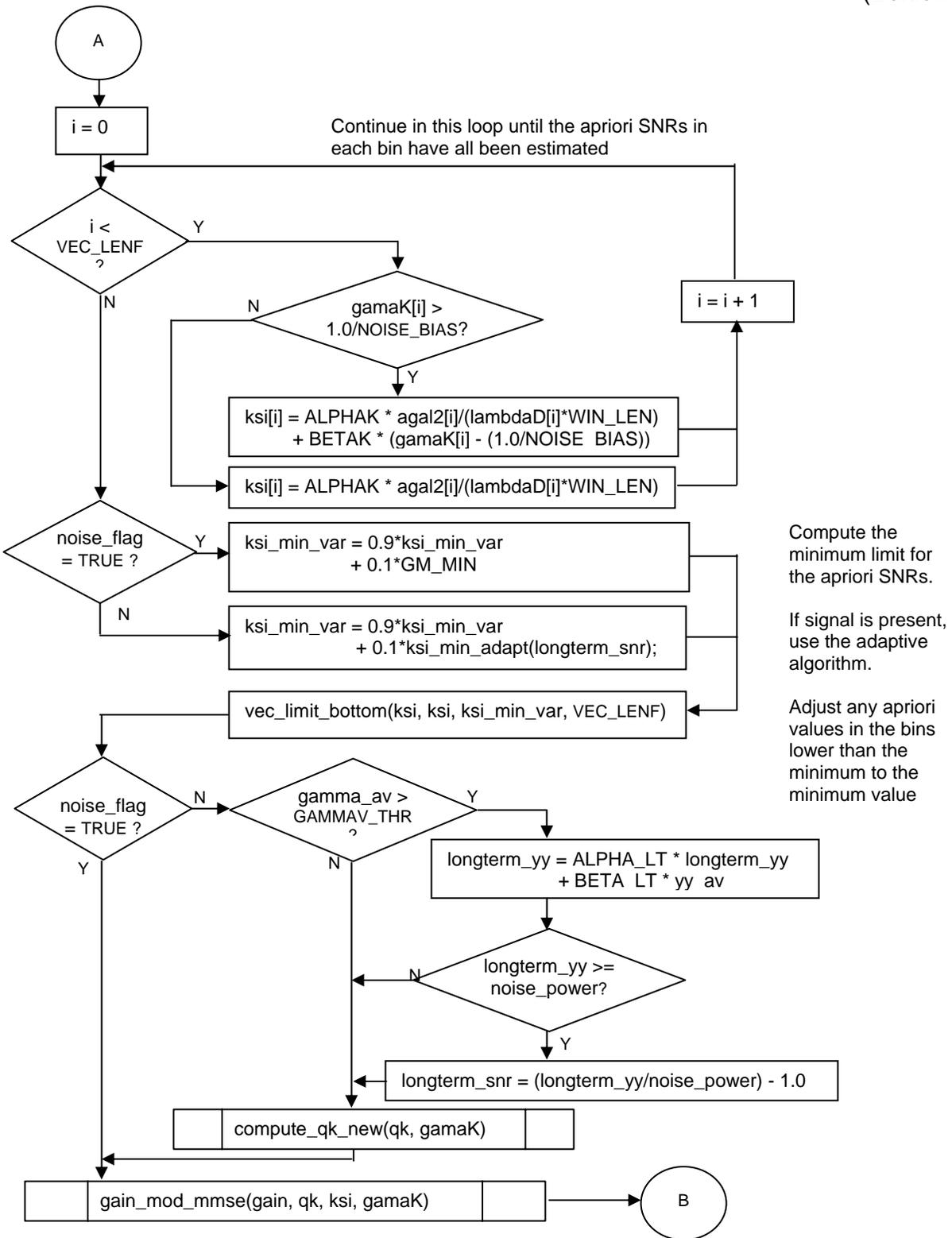
Figure E-4b. Process Frame (Part 2)
