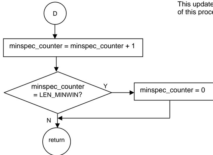
Figure E-6d. Processing to Search for Minimum PSD (Part 4)
