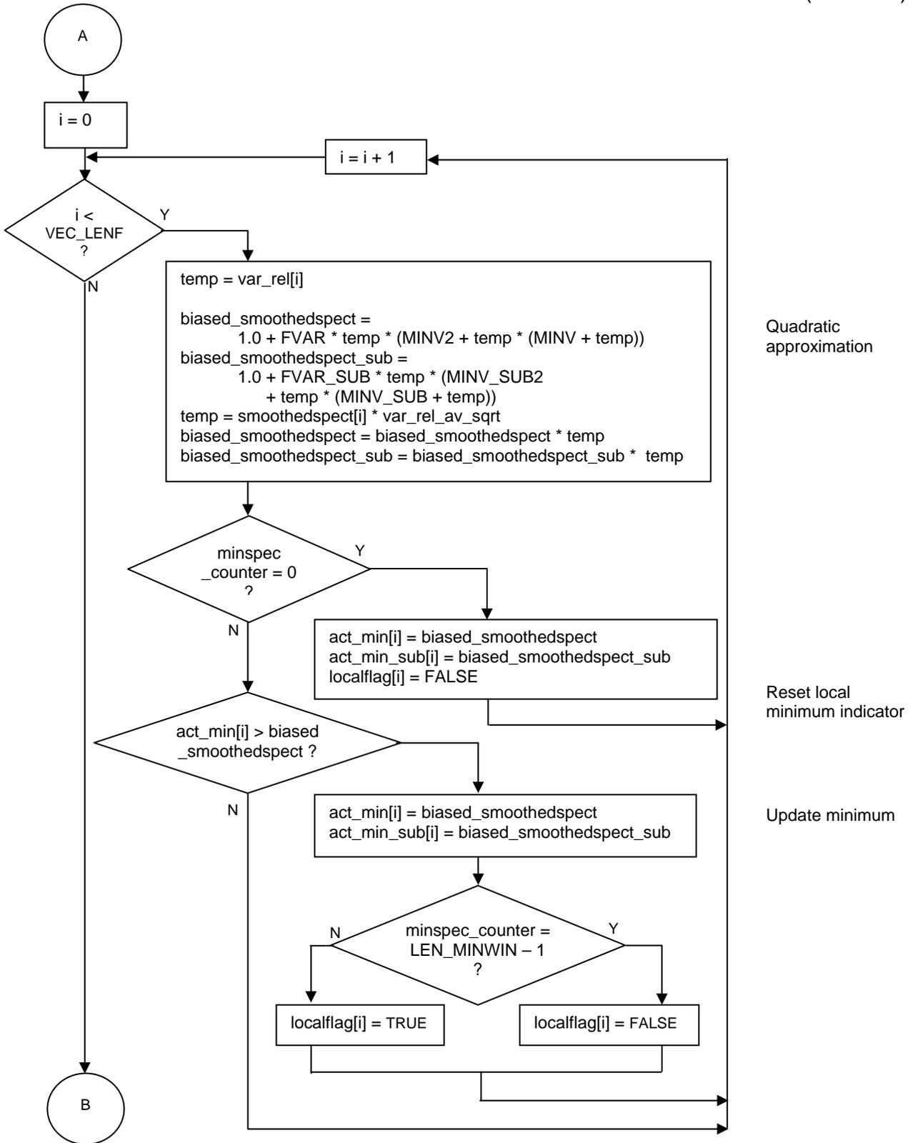
Figure E-6b. Processing to Search for Minimum PSD (Part 2)
