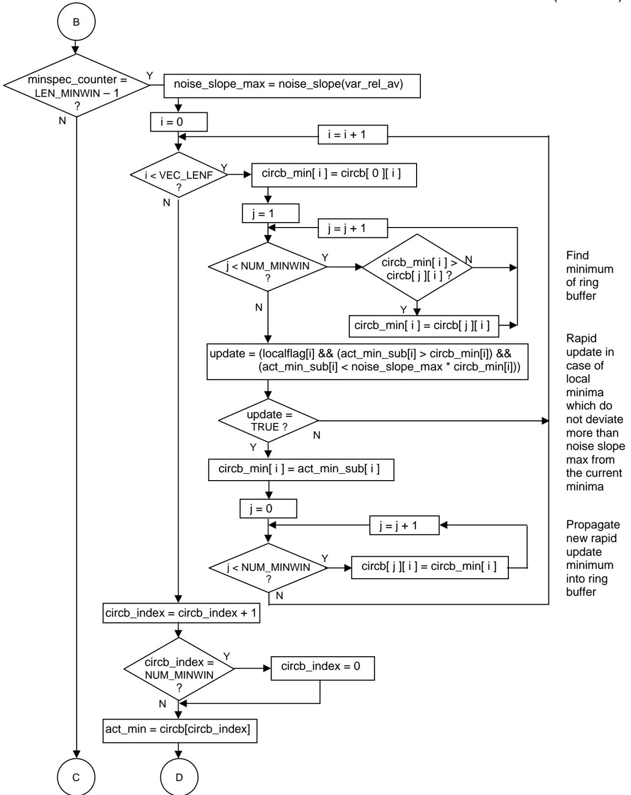
Figure E-6c. Processing to Search for Minimum PSD (Part 3)
