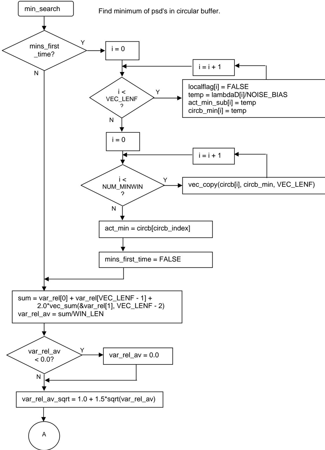
Figure E-6a. Processing to Search for Minimum PSD (Part 1)
