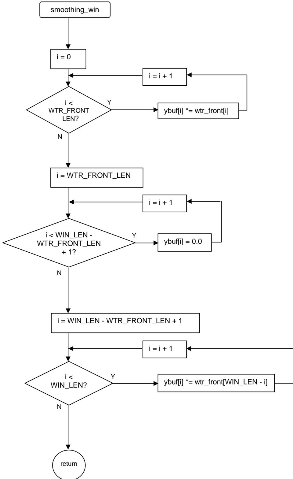
Figure E-12. Initialization of the Processing Buffer
