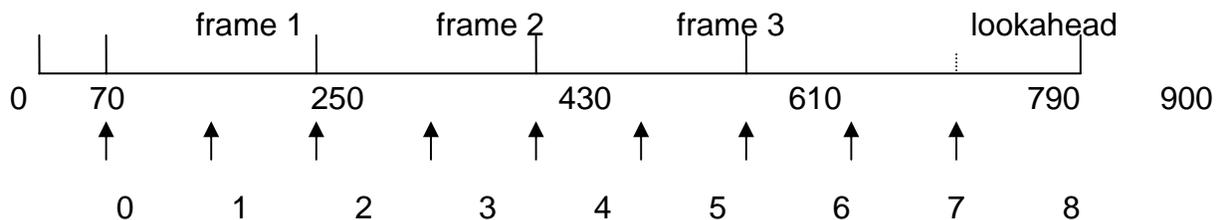
**Figure D-3. The computation positions of parameters for pitch smoother**
