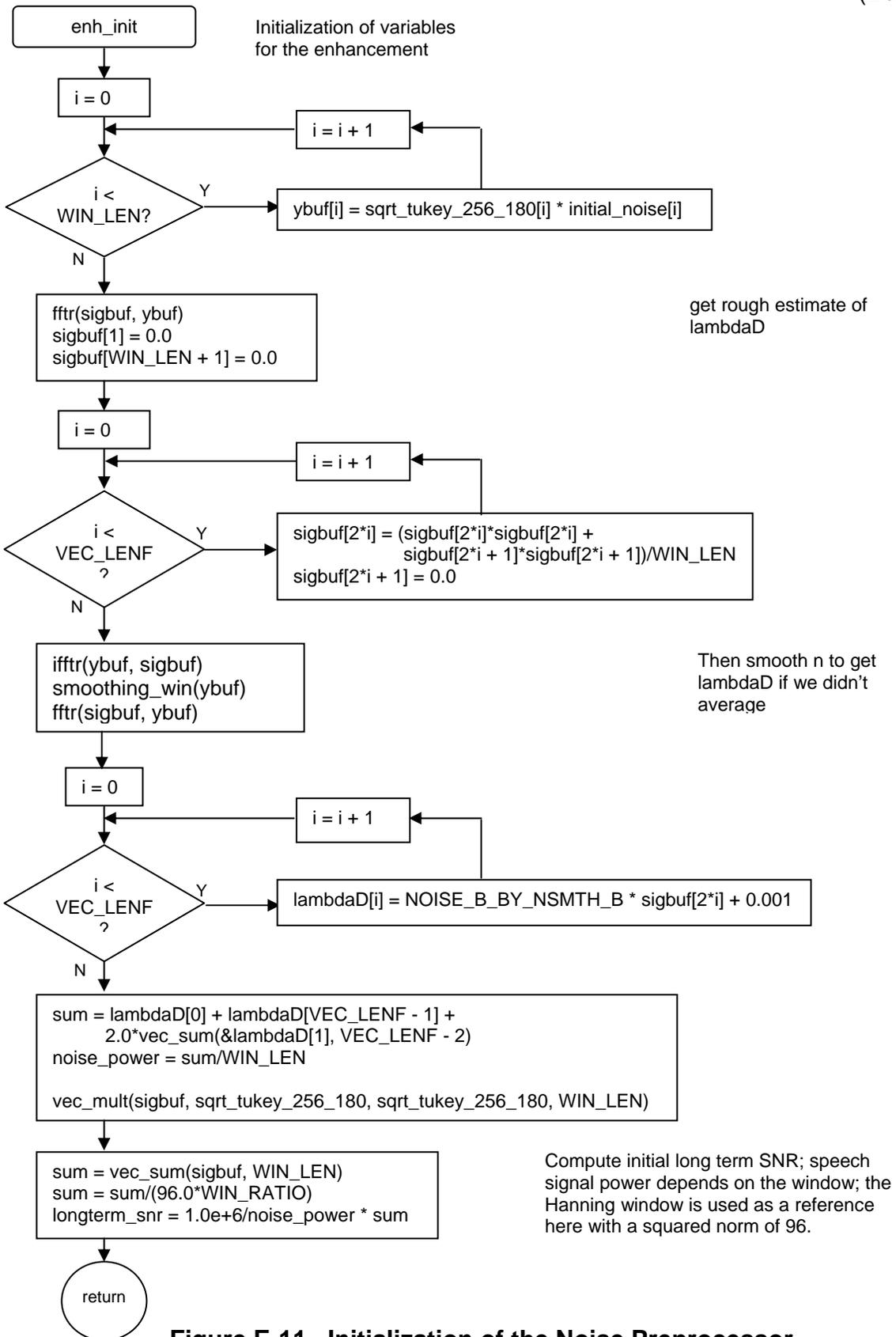
Figure E-11. Initialization of the Noise Preprocessor
