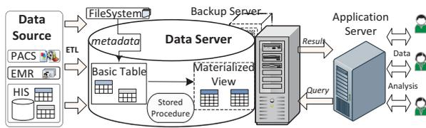
Fig. 1. The Initial Architecture of HEALTH Application
