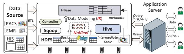
Fig. 3. The Architecture of HEALTH based on Hadoop Ecosystem
