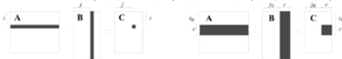
Figure 21.7: Matrix multiplication. Each element of C is computed from a row of A and a column of B . With blocking, a c \times c block of the C matrix is computed from a c \times N block of A and a N \times c block of B .
