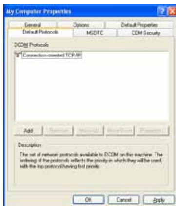
Image 7: In the Default Protocols tab, set the DCOM Protocols to “Connection-Oriented TCP/IP”.
