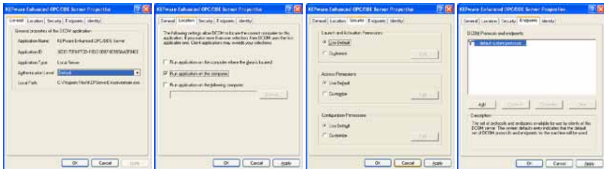
Image 11: The settings in the first four tabs (General, Location, Security, and Endpoints) should remain at their default settings as shown above.
