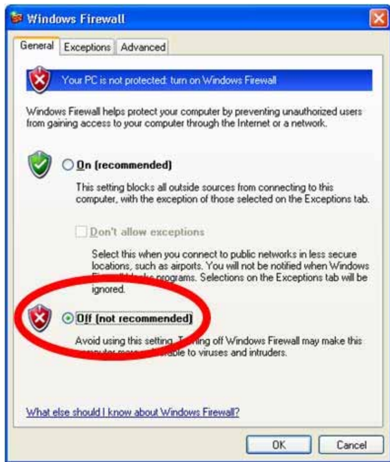
Image 3: Temporarily turn off the Windows Firewall to allow remote access to the OPC Server computer.
